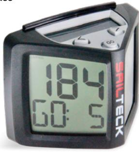
Sailteck powers up in **OUTDOOR** daylight when you **UNCOVER** the solar panel (if indoors, light the solar panel with a lamp or phone). Place on a table to turn off. Power-off is automatic when there is neither motion nor sun for 2 minutes.
